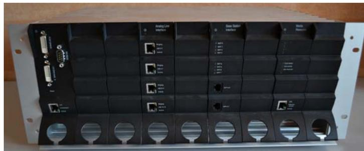
**Figure 3** Spectralink DECT Server 2500 Chassis with CPU (without Link option) and Interface cards
