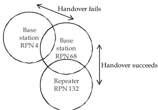
Also, a handset must never be able to detect two radio units (base stations or repeaters) with the same RPN at the same time. The handset will not be able to make a handover. If an RPN is reused, the units must be placed at a fair distance from each other.
