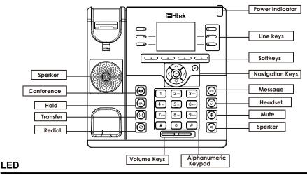
Power Indicator: Steady green when power on, blinking green when the call is ringing.
